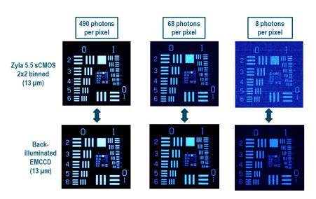
Images at a range of incident light intensity, acquired using backilluminated EMCCD iXon 888 and Zyla 5.5 sCMOS cameras (2x2 binned pixels). At low light intensities, the Signal to Noise Ratio advantage of the EMCCD is apparent
