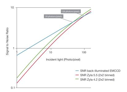
Plot of Signal to Noise Ratio versus Incident Photon Intensity, comparing back-illuminated EMCCD iXon 888 (13 µm pixel size) to 2x2 binned Zyla sCMOS cameras (13 µm pixel size after binning)
